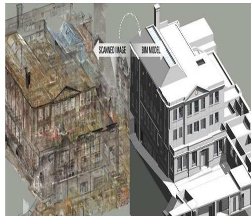
Laser scan is implemented on elements like exterior & interior walls, doors, windows, ceiling, curtain walls, floor, roof, major furniture & fixtures, structural column, wall, beam & slab, bracing, trusses, floor & roof framing, duct, pipes, cable tray, light fixture, electrical outlet and other equipment.
