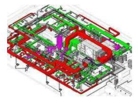
Mechanical ducting: Mechanical ducting system consist with the mechanical equipment like AHU, VAV, CU, FCU, RTU etc. with duct, duct fitting, hangers, dampers, access panel, access door, with all accessories.
